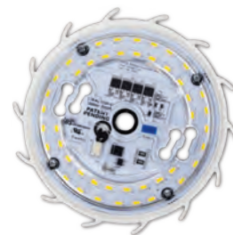
SL12-AC120R-W 14W, 1430LM, 3000K
